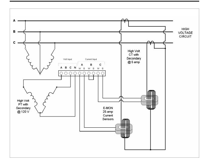
This special high voltage meter installation shows the correct wiring procedure for 3-wire high voltage circuits. In this application, the 2 element meter connection is used on the secondary circuits of the user supplied high voltage PTs and CTs.
